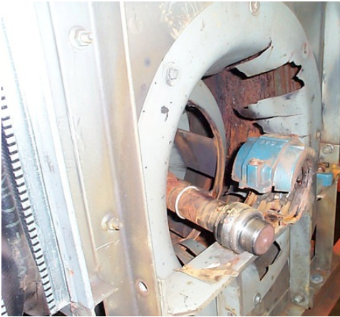
Fan & Motor Bearing Failures Can Be Prevented by Measuring Vibration
